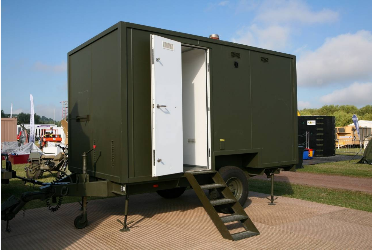
Trailer unit with toilet and wash facilities
